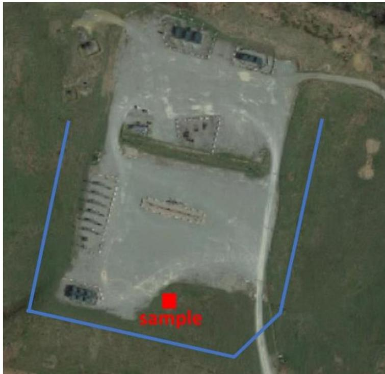
Figure 3. Aerial image of the DeArmitt pad. The red square marks the location of the air sample taken. The blue line shows the pathway for the walking survey for CH<sub>4</sub>. The aerial image is from Google Maps.
