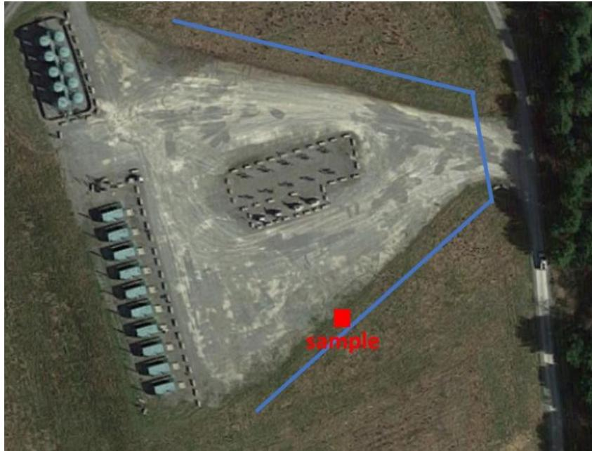
Figure 4. Aerial image of the Hutchinson pad. The red square marks the location of the air sample taken. The blue line shows the pathway for the walking survey for CH<sub>4</sub>. The aerial image is from Google Maps.
