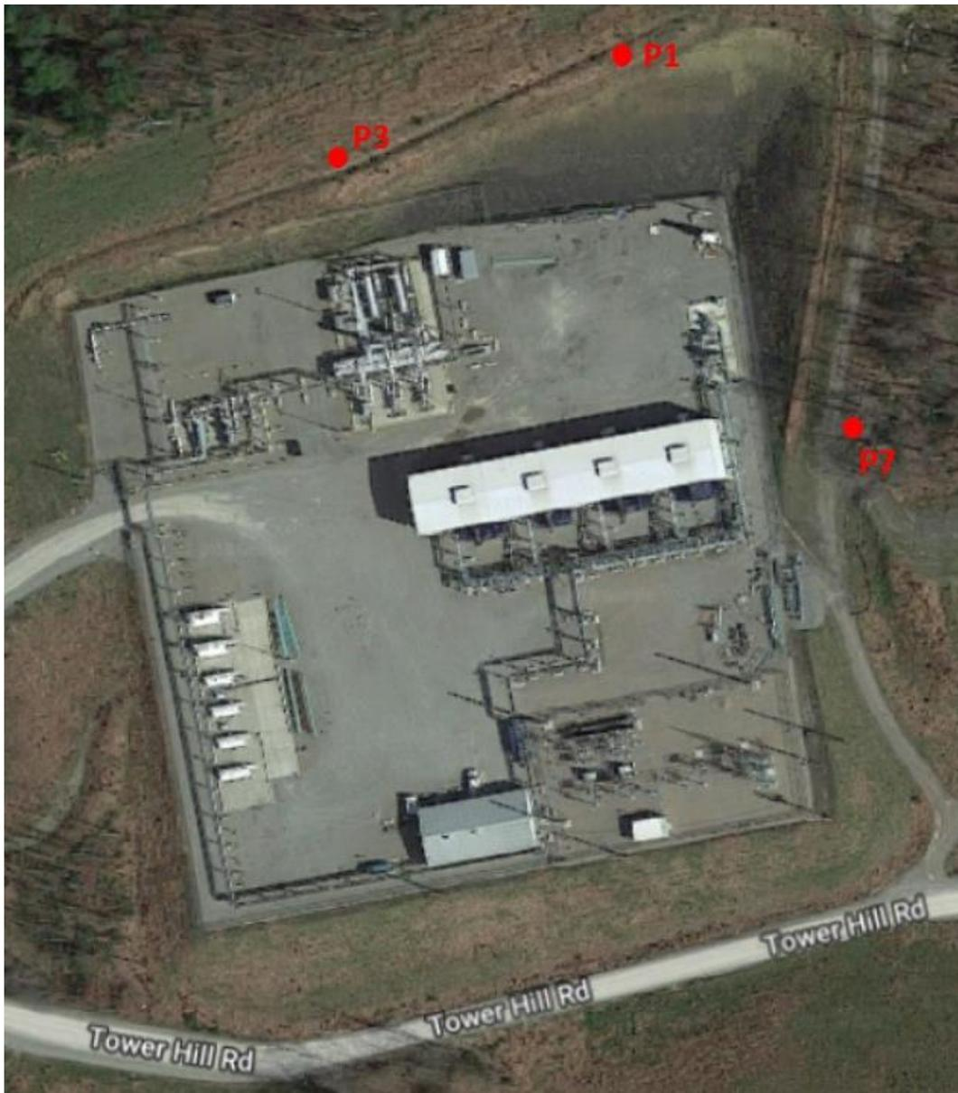
Figure 1. Aerial image of the Mamont compressor station. The red squares labeled P1, P2 and P7 mark the locations where carbon monoxide data loggers were collected and replaced. Air samples and hand-held sensor readings were taken at position P7; the temperature relative-humidity data logger was placed at P7. The aerial image is from Google Maps.
