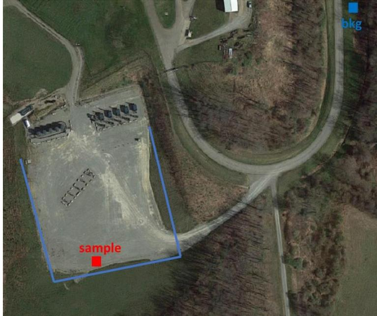
Figure 2. Aerial image of the Kuhns pad and nearby vicinity. The red square marks the location of the air sample taken. The blue line shows the pathway for the walking survey for CH<sub>4</sub>. The blue square labeled “bkg” marks the location of the background air sample. The aerial image is from Google Maps.
