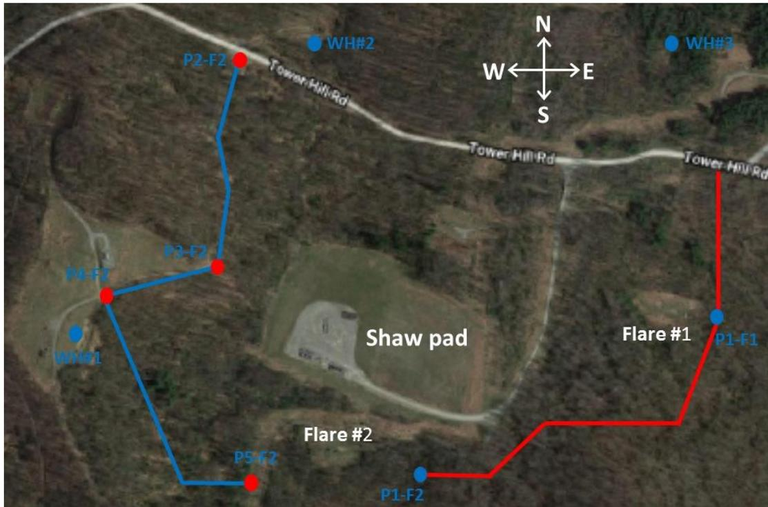
Figure 3. Aerial image of the Shaw pad and surroundings. Walking surveys for methane, sulfur dioxide and carbon monoxide were conducted on the red and blue paths on 7 and 10 February, respectively. Methane surveys at the well heads labeled WH#1, WH#2 and WH#3 were conducted on 10 February.
