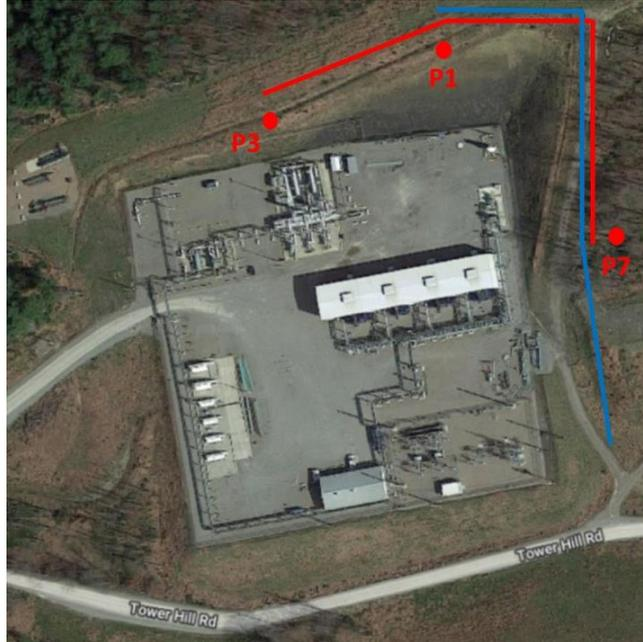
Figure 1. Aerial image of the Mamont compressor station. The red circles labeled P1, P2 and P7 mark the locations of carbon monoxide data logger placements. The red and blue lines show approximate paths of walking surveys for methane and sulfur dioxide surveys, respectively. The aerial image is from Google Maps.
