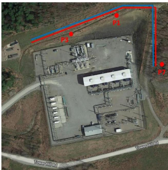
Figure 1. Aerial image of the Mamont compressor station. The red circles labeled P1, P2 and P7 mark the locations of carbon monoxide data logger placements. The red and blue lines show approximate paths of walking surveys for carbon monoxide and sulfur dioxide, respectively. The aerial image is from Google Maps.
