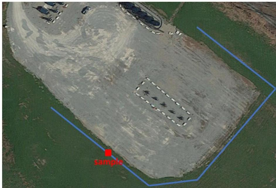
Figure 5. Aerial image of the Mamont pad. The red square marks the location of the air sample taken. The blue line shows the pathway for the walking survey for CH<sub>4</sub>. The aerial image is from Google Maps.
