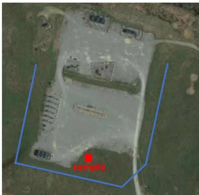
Figure 3. Aerial image of the DeArmitt pad. The red square marks the location of the air sample taken. The blue line shows the pathway for the walking survey for CH<sub>4</sub>. The aerial image is from Google Maps.
