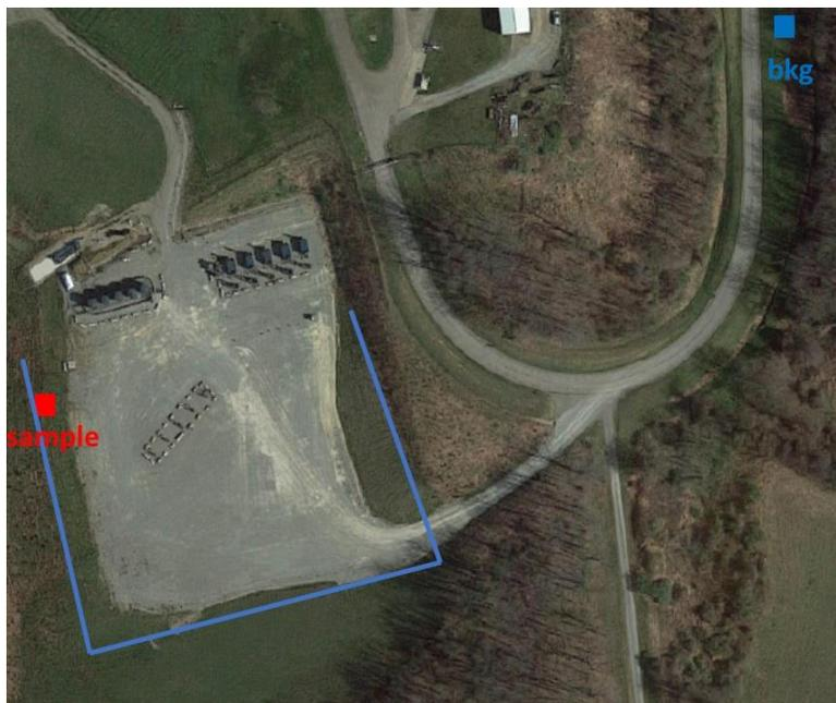
Figure 2. Aerial image of the Kuhns pad and nearby vicinity. The red square marks the location of the air sample taken. The blue line shows the pathway for the walking survey for CH<sub>4</sub>. The blue square labeled “bkg” at the upper right in the figure marks the location of the background air sample. The aerial image is from Google Maps.
