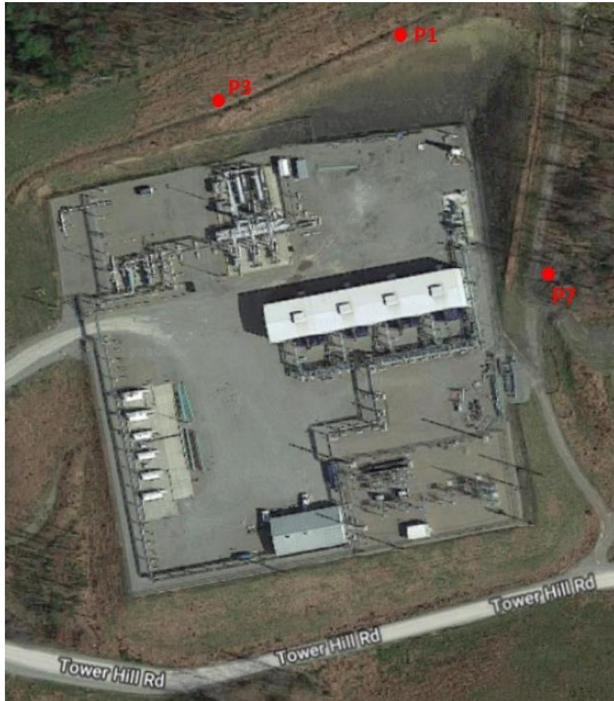
Figure 1. Aerial image of the Mamont compressor station. An air sample was taken at position P7. Hand-held sensor readings for CO, SO<sub>2</sub>, CH<sub>4</sub>, NO<sub>2</sub> and CH<sub>2</sub>O were recorded at P7. CO data loggers were placed at the positions P1, P2 and P7. The aerial image is from Google Maps.
