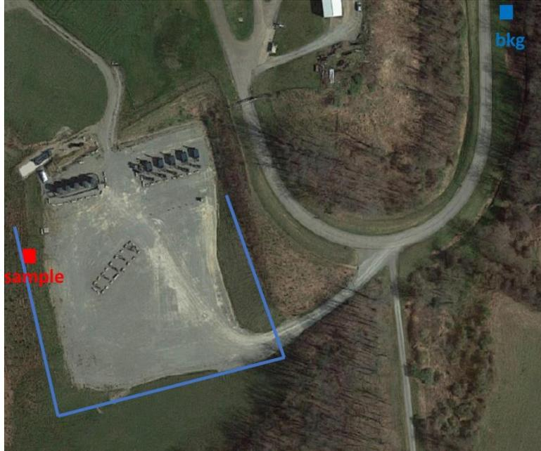
Figure 2. Aerial image of the Kuhns pad and nearby vicinity. The red square marks the location of the air sample taken. The blue line shows the pathway for the walking survey of CH<sub>4</sub>. The blue square labeled “bkg” at the upper right in the figure marks the location of the background air sample. The aerial image is from Google Maps. The distance from the location of the background sample to the Kuhns well head is about 200 meters.
