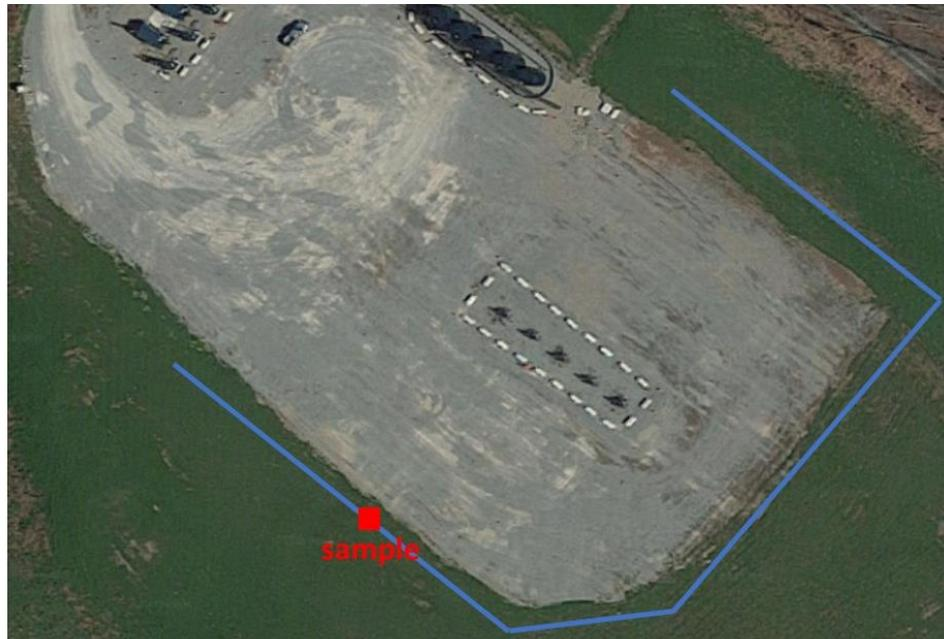
Figure 5. Aerial image of the Mamont pad. The red square marks the location of the air sample taken. The blue line shows the pathway for the walking survey of CH<sub>4</sub>. The aerial image is from Google Maps.
