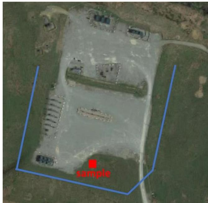
Figure 3. Aerial image of the DeArmitt pad. The red square marks the location of the air sample taken. The blue line shows the pathway for the walking survey of CH<sub>4</sub>. The aerial image is from Google Maps.
